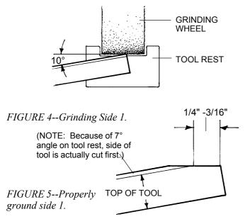
Move the blank back and forth across the face of the wheel until you have ground a 10° angle on approximately 3/16"
