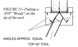
This means that if you set the tool flat on the tool rest the tool rest angle would have to be increased to get an even flat. This wouldn't be worth the effort, so the easy way is to free hand it. I always start by touching the heel of the tool first, and then change the angle until a slight flat is put on the tip. Of course, the angle you're holding it at has to be close when starting to get desired results.
